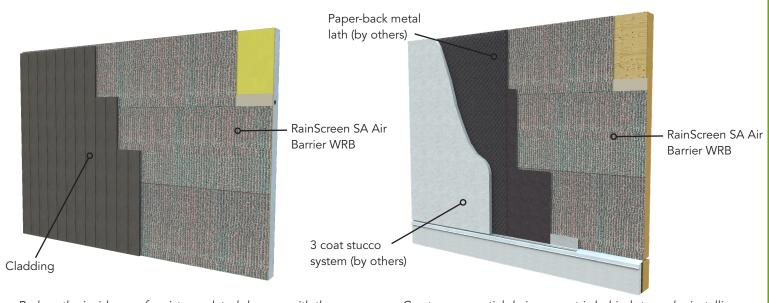
Reduce the incidence of moisture related damage with the all in-one air barrier, WRB rainscreen system, RainScreen SA, behind the cladding system. Create an essential drainage matrix behind stucco by installing RainScreen SA. No change to design or installation practices is required.
