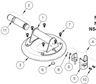
\* Repair Kit 90504 for Metal Cups (6, 8, 9 and Plunger Lube)
