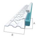
1/4" removable leg provides a clean, stucco-free caulk gap. A clean 1/4" x 1/4" caulk gap assures the most efficient caulk seal for optimal moisture protection.
