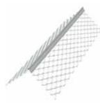
Clark Dietrich 1A expanded flange corner bead is used to provide strong corner reinforcement for conventional plaster applications. A solid metal nose provides a straight, rigid ground for screeding, and the 2-7/8" or 3" flanges can be flexed easily over irregular, uneven surfaces. Plaster keys near the solid nose provide increased reinforcement where needed and ensure straight corners.
