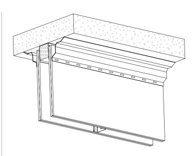
Profile fastened to wall surface using nom. 1/2" (13mm) steel staples spaced nom. 8" (203mm) OC. See UL System for more detail.
