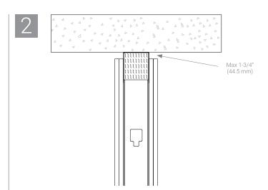
Max 1-3/4" (44.5 mm) wide joint between gypsum layer(s) and bottom surface of floor/deck.
