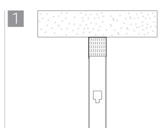
Mineral wool block compressed into ceiling runner and secured in place using cup head weld pins. See UL System for more detail
