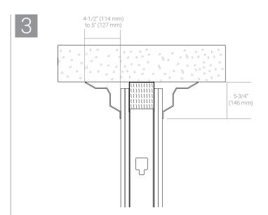
Place SFJP80 profile over joint on both sides of wall. Leg of Joint profile offset nom. 5-3/4" (146mm) from underside of floor/deck. Opposing leg offset from face of steel ceiling runner 4-1/2" (114mm) for 1Hr and 5" (127mm) for 2 Hr configurations. See UL System for more detail.
