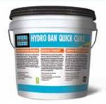
A rapid, thin, liquid applied ready-to-use waterproofing membrane that is ANSI A118.10 Compliant. Featuring Wet-Cure technology, this allows curing even in humid, cold and damp environments. HYDRO BAN® Quick Cure allows for flood testing in as soon as 30 minutes<sup>4</sup> allowing contractors to install a shower system all in one day.
