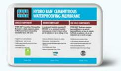
A one component, polymer fortified, cement based waterproofing material that mixes only with water. HYDRO BAN Cementitious Waterproofing Membrane handles negative and positive hydrostatic pressure up to 2 BARS (29 PSI (.2 MPa)) when applied at 40 Mils (1 mm) thick. Flood test within 2 hours. Passes ANSI A118.10 Waterproofing and ANSI A118.12 Crack Isolation (with mesh/fabric up to 1/8" (3 mm).
