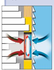
Self-adhered – Being fully adhered and nail sealable, Blueskin® VP100 is more effective than traditional house wraps at preventing the movement of air and moisture through walls.
