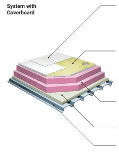
MECHANICALLY ATTACHED OR FULLY ADHERED SINGLE-PLY MEMBRANE
