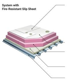
TPO OR PVC MECHANICALLY ATTACHED WHITE SINGLE-PLY MEMBRANE
