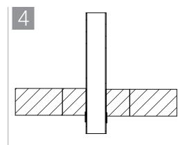
Remove form once mortar has fully cured.
