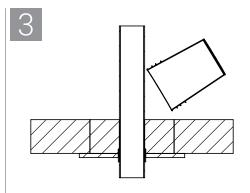
Mix mortar with water. See mortar bag label for additional instructions. Pour mortar and allow to cure.
