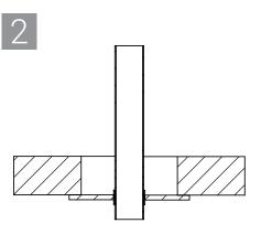
Place wrap strip around combustible penetrant. Refer to UL system for wrap strip laters and position.
