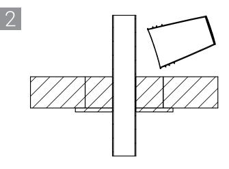
Mix mortar with water. See mortar bag label for additional instructions. Pour mortar and allow to cure.
