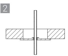
Place collar around combustible penetrant per UL system.
