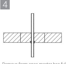
Remove form once mortar has fully cured.
