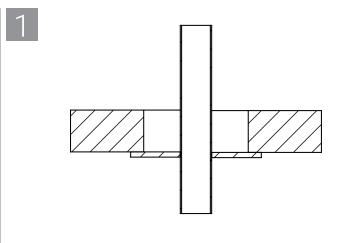
Place temporary form on the bottom side of wall or floor. This will hold your mortar in place. Note: use non-moisture absorbing material.
