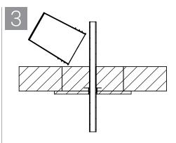
Mix mortar with water. See mortar bag label for additional instructions. Pour mortar and allow to cure.
