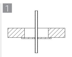
Place temporary form on the bottom side of wall or floor. This will hold your mortar in place. Note: use nonmoisture absorbing material.
