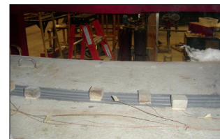
Thermocouples register no more than 248°F (120°C)
