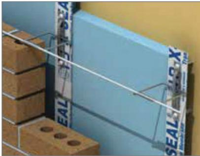
**Dimensions:** Available in leg lengths from 1/2" - 4-1/2" to accommodate wallboard and/or insulation
