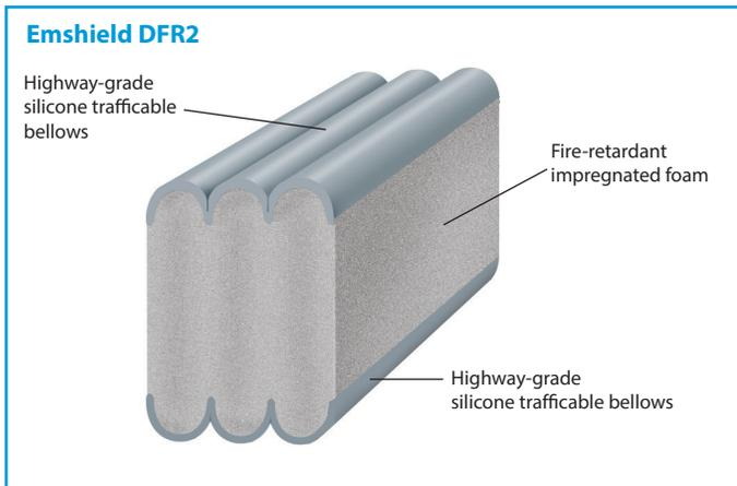
Emshield DFR2 builds on EMSEAL's track record of over 30 years of innovation in sealing structural expansion joints with impregnated foam sealants.
