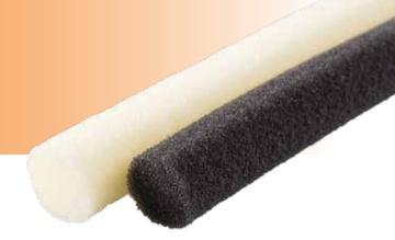
OCFoam<sup>TM</sup> is a an open-cell polyurethane foam backer rod used as a backing in concrete construction for elastomeric and other hot-pour and cold-applied sealants. OCFoam acts as a barrier, limits the depth of sealant required and prevents excessive sealant use.
