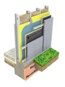
For open joint rainscreen applications, EnergyShield CGF Pro offers a black facer, eliminating the need for a black out fabric.
