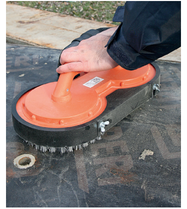
Cleaning formwork units
