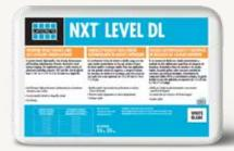
A cement-based, high quality, fast drying dual purpose selfleveling underlayment/interior decorative wear surface topping. For application over a wide variety of substrates including concrete, VCT, and tile. Can be placed from 1/16" to 1-1/4" (1.5 - 32 mm) in a single lift.
