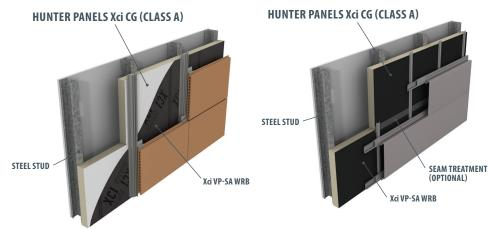
\*The location and number of WRBs in the wall assembly are determined by the architect. Contact Hunter Panels for a list of approved WRBs for NFPA 285 compliance.
