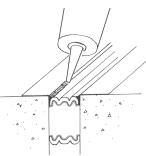
• Where WFR foam meets at butt joins, tool the excess silicone that squeezes out from the top and between the bellows.
