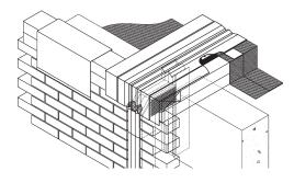
Like the solid-wall closure, the cavity-wall RoofJoint closure, is a factory-fabricated transition piece made from Seismic Colorseal. The difference is an extended, horizontal setback portion of coated foam to bridge the cavity from facade to structural backup wall. The sides of the "bridge" are additionally coated with silicone to seal them against
