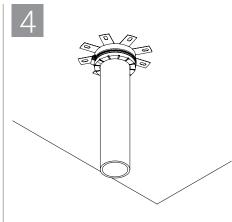
Fold Retaining tabs toward penetrant and mounting tabs away from penetrant.
