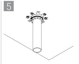
Slide collar to tightly abut assembly surface. Mechanically fasten collar mounting tabs to assembly surface. Number of tabs and fastener requirements per appropriate UL System
