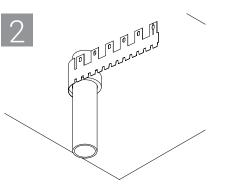
Encircle Wrap strip layers with retraining steel having a 1" lap. See Product Data Sheet for appropriate steel Restraining collar material
