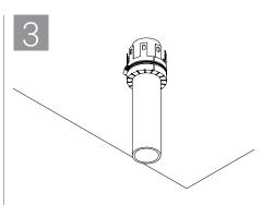
Hold collar material in place using steel hose clamp. Hose Clamp positioned at mid height of each wrap strip stack
