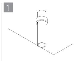
Apply Wrap Strip around penetrant, ends held together with foil tape. See appropriate UL System for required number of wrap strip stacks and layers.
