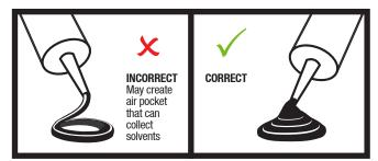
Do not apply mastics in a circle where an air pocket could collect solvents and possibly extract material that could be damaging to the mirror. The best way to apply Extra/Build<sup>®</sup> from a cartridge is to start from the center and let the mastic naturally expand out as it's being gunned.
