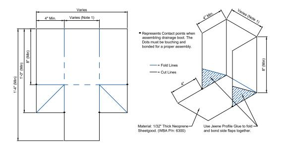
1. Overall width of Boot Transition will be determined on the amount of movement the WSW system can accommodate during normal movement ranges. WBA suggests that the dimension will be at least Maximum Opening plus 1". This is to ensure that there will not be any damage to the boot while the system is at maximum opening.
