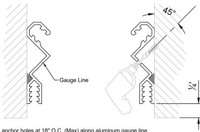
3 - Field drill anchor holes at 18" O.C. (Max) along aluminum gauge line. Drill through aluminum into adjacent construction.
