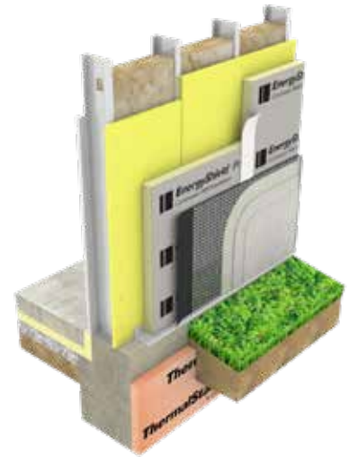
Steel studs, batt cavity insulation, glass-mat faced sheathing, EnergyShield Pro with taped joints, grade D building paper, expanded metal lath, cement plaster scratch and brown coats, stucco finish.
