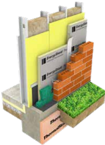
Steel studs, batt cavity insulation, glass-mat faced sheathing, EnergyShield Pro with taped joints, mortar net, brick.
