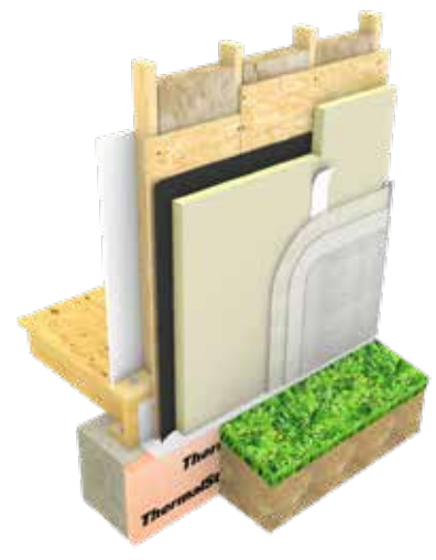
Wood studs, batt cavity insulation, wood sheathing, water resistive membrane, EnergyShield Stucco-Shield, basecoat, mesh, acrylic finish.
