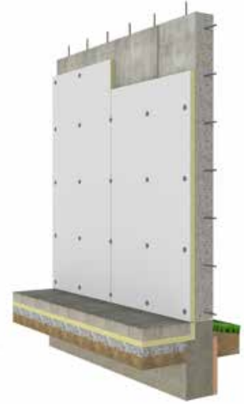
Concrete: Tilt-Up Wall or Residential Basements
