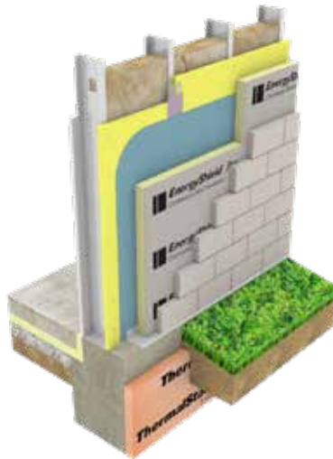
Steel studs, batt cavity insulation, glass-mat faced sheathing, liquid applied air and moisture barrier, EnergyShield Pro, stone cladding.
