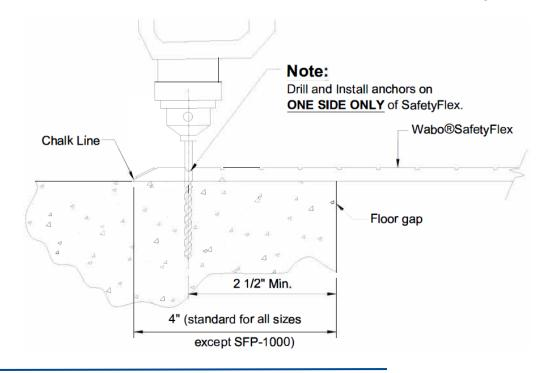
To allow for thermal expansion of the EPDM Rubber cover, leave a 1/8" approximate gap between Wabo®SafetyFlex sections.
