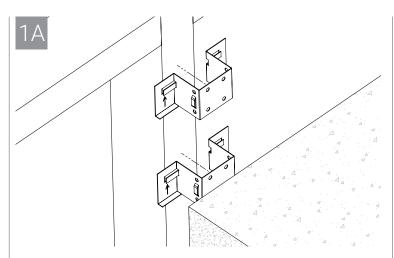
Clip U-Bracket onto mullions (vertical framing) nominally 2" (51 mm) from bottom of sill, flush with the bottom of the floor and 2" (51 mm) from the top of the transoms (horizontal framing) below the floor. U-Brackets lock into place with a strike of a mallet.
