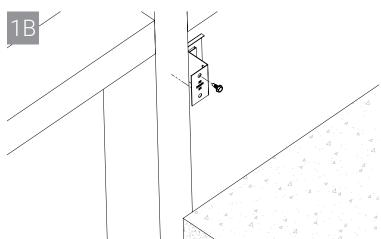
Attach Z-Bracket to mullion (vertical framing) using minimum of one No. 10 by min 1/2" long self-drilling, self-tapping steel screw or as specified in the applicable UL System. Z-Bracket to be located nominally 2" (51 mm) from bottom of sill and 2" (51 mm) from of the top of the transoms (horizontal framing) below the floor.
