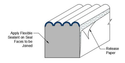
Install the material, starting at one end of the joint working towards the other end of the joint. Make sure not to pull, twist or stretch the material in the process of installation.
