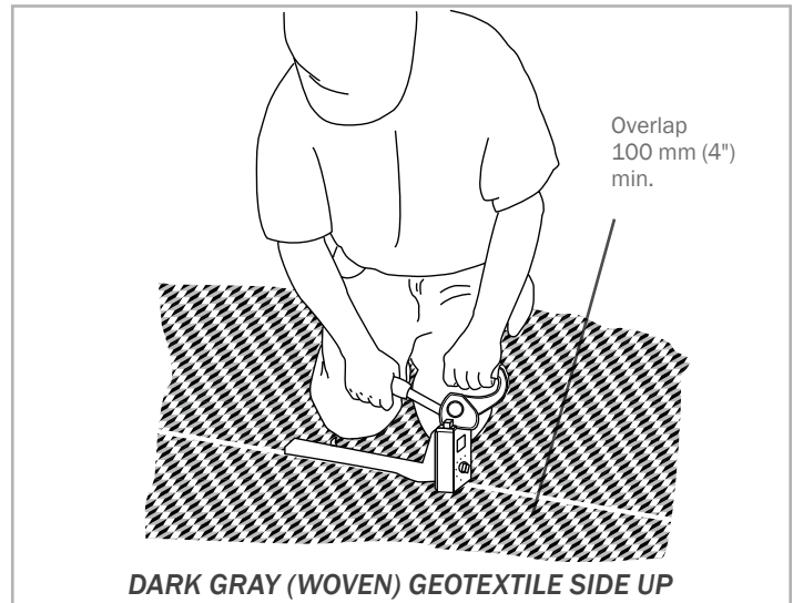
Figure 1.2 – Secure overlaps together with fasteners
