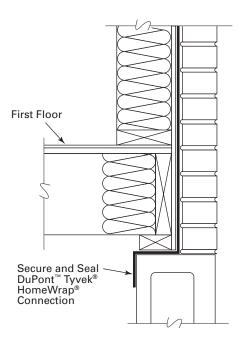
To ensure continuity of the air barrier membrane from the bottom of the wall into the interior, install the **Tyvek® WRB** as shown above. Use Method 2 for slab on grade applications.
