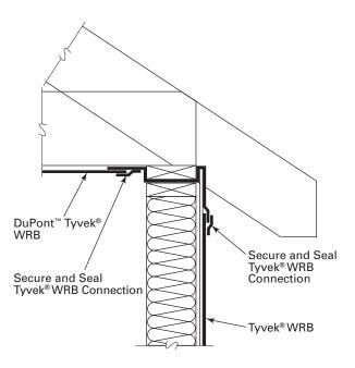
To ensure continuity of the air barrier membrane from the top of the wall to the interior, install the **Tyvek® WRB** as shown above.
