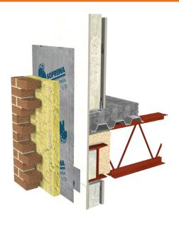
SOPRASEAL® Stick VP is a self-adhered vapor-permeable air barrier membrane used in wall construction. SOPRASEAL Stick VP is composed of a tri-laminate polypropylene composite facer coated with a high tack self-adhesive backing protected by a silicone release film. The self-adhesive properties of SOPRASEAL Stick VP are unmatched in the industry, and the roll size combined with high tack adhesive make it very easy to install.
