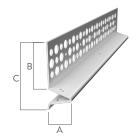
Designed to direct moisture from the stucco and to act as a stop. Install on masonry construction where stucco and foundation walls meet.
