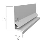
Designed to provide a flashing transition from stucco, siding, stone over a brick ledge, at a wall transition.
