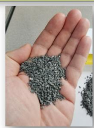
BASF Masterseal 940 50lb Bag (22.68Kg) (P/n: #33137) for broadcasting onto Wabo®Crete Parking Series Elastomeric Concrete exposed surface.
