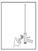
apply petroleum jelly on the inside threads of the basket. This allows for easy can After cleaning the gun basket with solvent, Page 3 of 3
