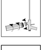
When the can is empty, remove the can by turning counter clockwise. A small amount of foam will be present in the gun basket.
