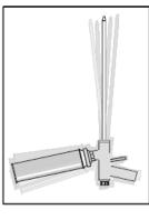
When reusing after short periods of storage, simply shake the gun and can unit for 1 minute.
