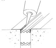
• Where DFR foam meets at butt joins, tool the excess silicone that squeezes out from the top and between the bellows.
