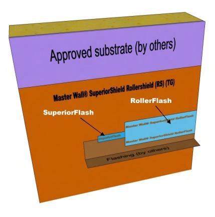
Typical Seam Sealing; 2" (50 mm) each side of joint or transition
