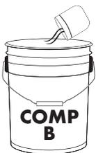
**2.** Pour 2/3 liquid Component-B into a clean container. Add 2K/M powder (Comp-A) and mix to a lump free creamy consistency with a strong, slow speed (300 rpm) mechanical mixer.
