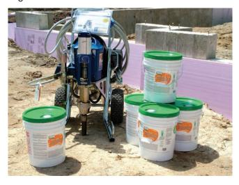
The Graco heavy-duty texture gun is recommended for use with the following tips: For best results, use the 0.051" (Graco GHD551) heavy-duty switch tip. For spraying of primer coat, a smaller orifice tip such as the 0.035" (Graco GHD635) can be used. Tips should be reversible types for easy clean out. For more complete spraying equipment information, please view INSTALLATION INSTRUCTIONS: SPRAYER EQUIPMENT GUIDELINES FOR W. R. MEADOWS FLUID-APPLIED MEMBRANES available at www.wrmeadows.com.
