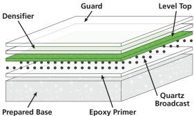
Minimum placement thickness for polishing applications is 3/8" (9.52 mm). Minimum placement thickness for non-polished topping applications is 1/4" (6.35 mm). Minimum placement thickness for non-polished underlayment applications is 1/8" (3.18 mm). This product can be feathered at the edges to meet adjacent floor elevations in underlayment applications. For all applications, the maximum non-extended placement thickness is 2" (50.8 mm) neat and 3" (76.2 mm) when extended with aggregate.
