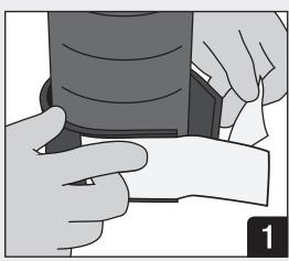
Measure and cut Tuck-In Wrap Strip to appropriate length (or use pre-cut wrap strips) for pipe size and layers required as per system specifications.
