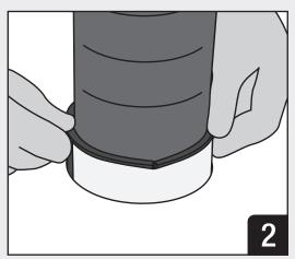
Wrap Tuck-In around pipe and position according to system requirements. Secure with provided adhesive installation tab or equivalent.
