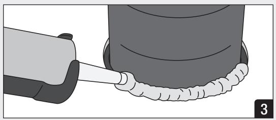
Seal the system with 3M™ Fire Barrier Sealant applied to appropriate interfaces as per system specifications.
