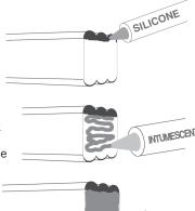
IMPORTANT: All sticks of DFR3 foam MUST have a coating of intumescent on the faces of all joins. This ensures that joins do not compromise the fire barrier.
